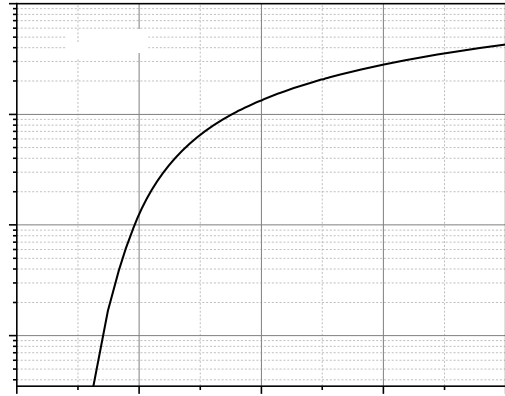
Figure 8. Forward characteristic of body diode
